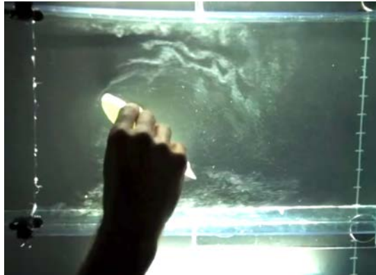
Fig. 6: A water tunnel visualization where a wing model can be rotated to examine the impact of orientation on aerodynamism [32]. Here the physical referent is the wing and the physical presentation is the set of water bubbles.
