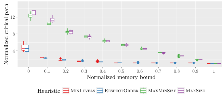
Figure 16: Critical path length obtained by each method for the MONTAGE dataset. The critical path plotted is divided by the original critical path. A memory bound value of 0 corresponds to the memory used by a DFS schedule, and a memory bound value of 1 corresponds to the maximum peak memory of the original graph.
