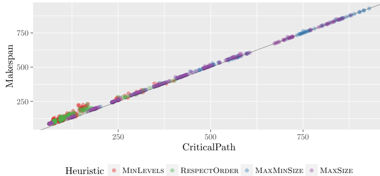
Figure 18: Makespan in function of the critical path length obtained by each method for the MONTAGE dataset.
