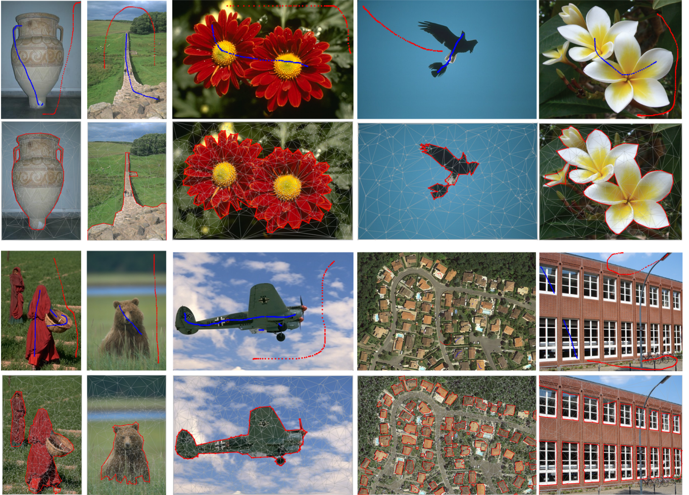
Fig. 13. Object contouring on a few example images. Our Delaunay point process samples polygons that capture the silhouettes of foreground objects. The user first draws a few scribbles that roughly characterize the objects of interest (blue lines) and the image background (red lines). Output polygons preserve details, such as the flower petals and the vase handles, while having low complexity.
