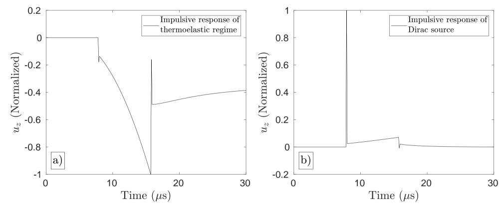
a): laser-generated seismic source under thermoelastic regime with displacements computed by combining the wave equation and the thermoelastic equations [2, 3, 5]. b): laser-generated seismic source under ablation regime which is modelled as a point-source [1, 2].
