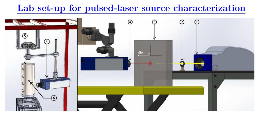
Two different experimental tools were mounted to investigate in Cartesian coordinates or in cylinder coordinates. ①: Q-Switched laser generator; ②: convergent lens; ③: Aluminium cuboid samples of various thickness (10, 50, 100 mm),  $V_p \approx 6350$  m/s,  $V_s \approx V_p/2$ ; ④: single point Laser Doppler Vibrometer (LDV); ⑤ core sample; ⑥ piezoelectric source.
