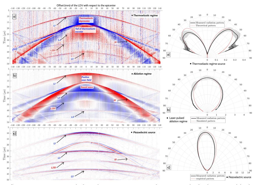
Seismogram measured along linear receivers on the 50 mm thick aluminum block with different sources, accompanied by simulated/modelled radiation patterns. a): radiation pattern of a point source (laser ablation); b): radiation pattern of a piezoelectric source ( $\Phi \approx 10 \text{mm}$ ); c): radiation pattern of a typical thermoelastic source [4] under laser irritation.
