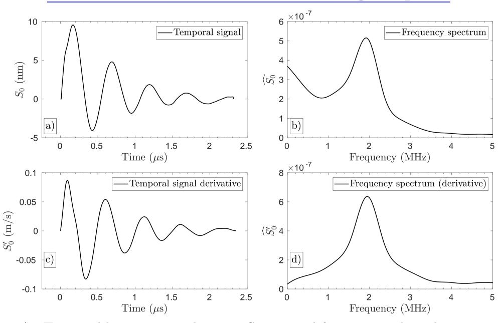
a): Temporal laser-generated source  $S_0$  retrieved from a record on the 50 mm thick aluminum block. b): Frequency spectrum  $\widehat{S_0}$  of the same source. c) First order time derivative of  $S_0$ , thus showing the surface vibration velocities. d) Frequency spectrum of  $S'_0$ .
