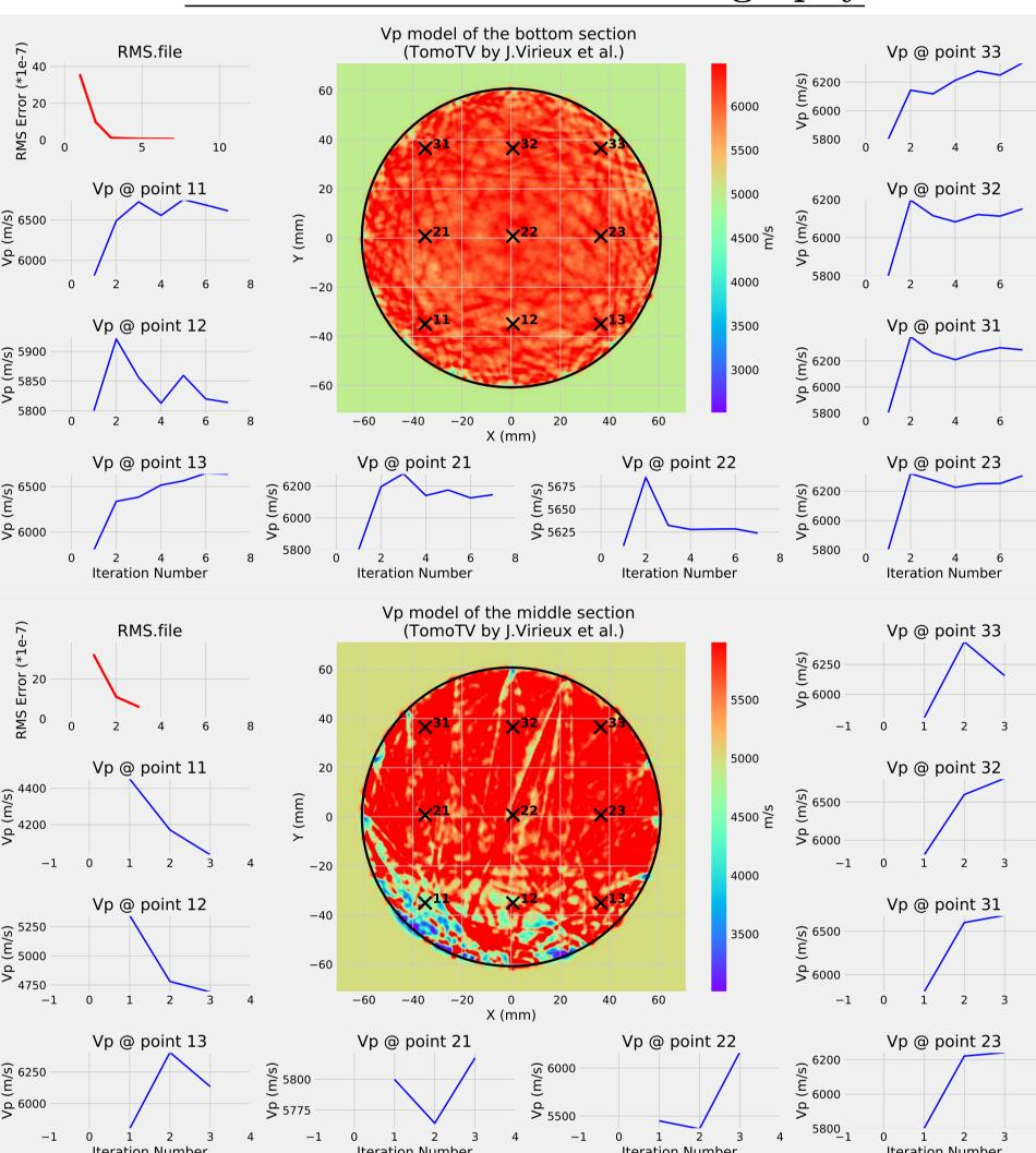
Considerable diffractions caused by the cavity disturbs heavily the first arrival time  $(2^{nd})$ . The first break based inversion algorithm doesn't take into account this complicated phenomenon leading to noisy, unstable and hardly convergent results.
