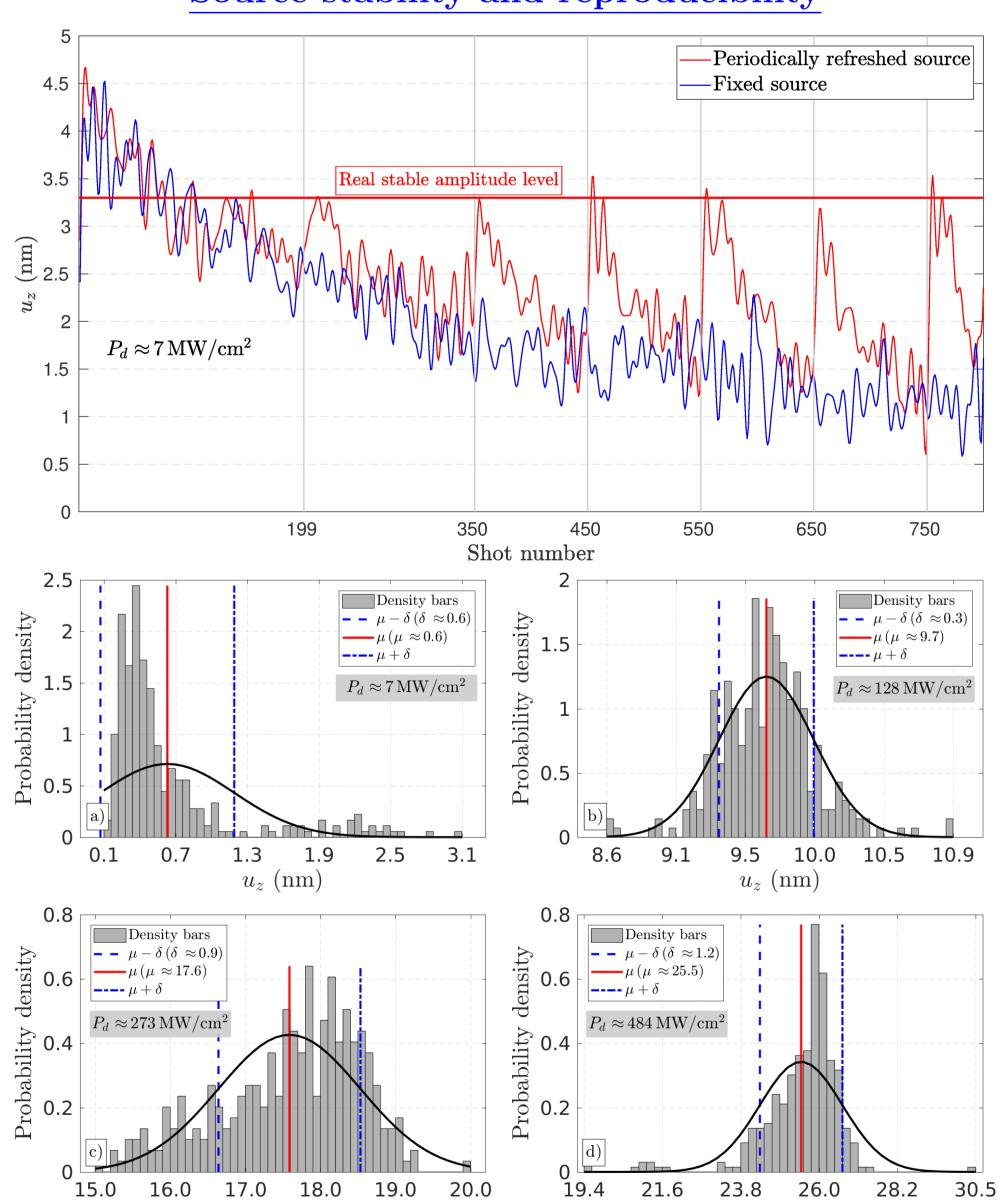
Distribution of first arrival seismic wave amplitudes  $u_z$  measured by LDV at the epicenter of the 10 mm thick aluminum block.  $P_d$  denotes the incident power density.
