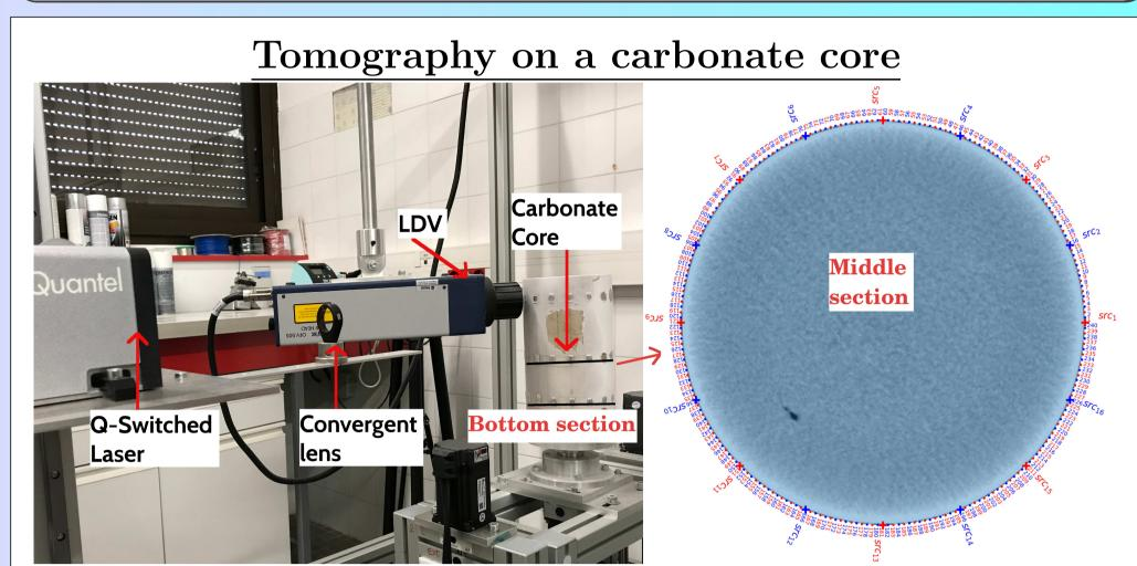
Application of the pulsed-laser ablation source on a carbonate core ( $\Phi \approx 120mm$ ). We used the point-source point-receiver setup. 16 sources (aluminum flakes) are uniformly distributed along the circumference of each normal section. Each source covers 300° (101 receivers @ 3°) in a symmetric manner. Thousands of shots are received by each source flake due to averaging recording.
