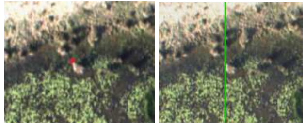
Fig. 13. The epipolar geometry of the optimized stereo calibration in flight. A selected pixel location in the front camera (left), and its corresponding epipolar line in the rear camera (right), showing the correctly aligned epipolar geometry.
