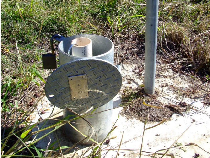
Figure 89. Monitoring bore with automatic pressure transducer. Bore is locked so that the automatic pressure transducer is not accessible during the measurement.
