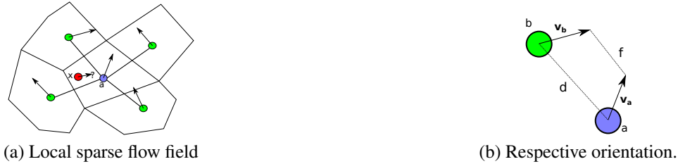
Fig. 2. Interpolation of flow vector at x (in red) according to the central flow vector (in purple) and the neighbouring flow vectors (in green). The purple and green points are the centers of their respective superpixels delineated by black lines.
