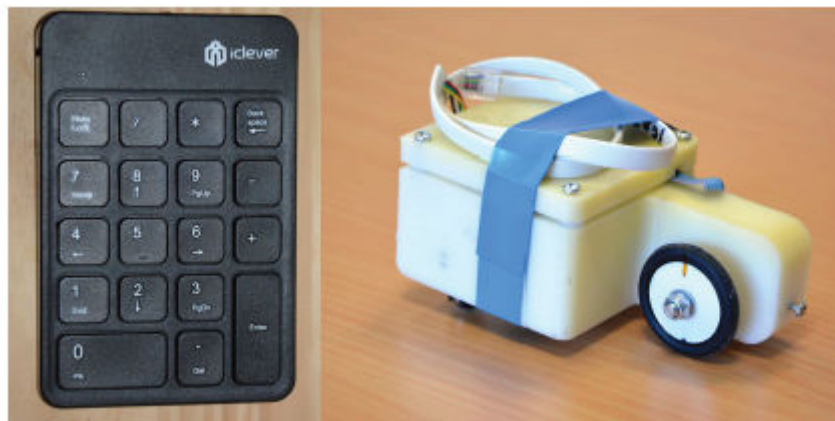
Figure 1. Morphorider and the wireless keypad used for marking nodes during acquisition.
