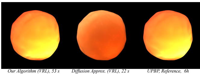
Fig. 21. Comparison between extended precomputed table (including double scattering) and diffusion approximation in VRL and UPBP as a reference on the Bumpysphere Scene. Material: Bumpysphere, g = 0.9 .
