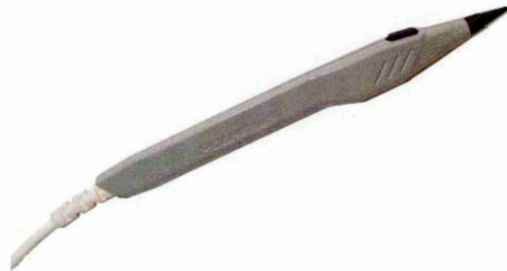
Figure 3.8 The Polhemus digital stylus.
