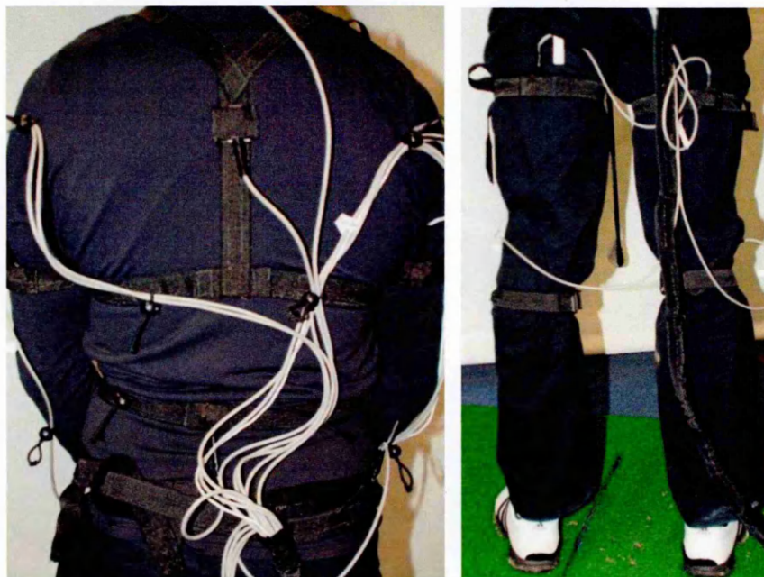
Figure 3.6 Electromagnetic sensors attached using: left – baselayer jacket with adjustable straps, right – adjustable leg straps.
