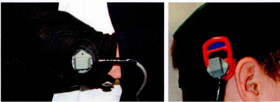
Figure 3.7 Electromagnetic sensors attached using: left – golf gloves, right – cap.
