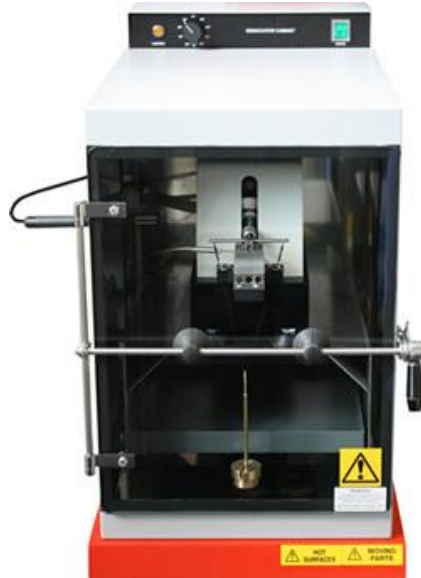
Figure 3.4-HFRR Atmosphere Control Cabinet (PCS Instrument Company)
