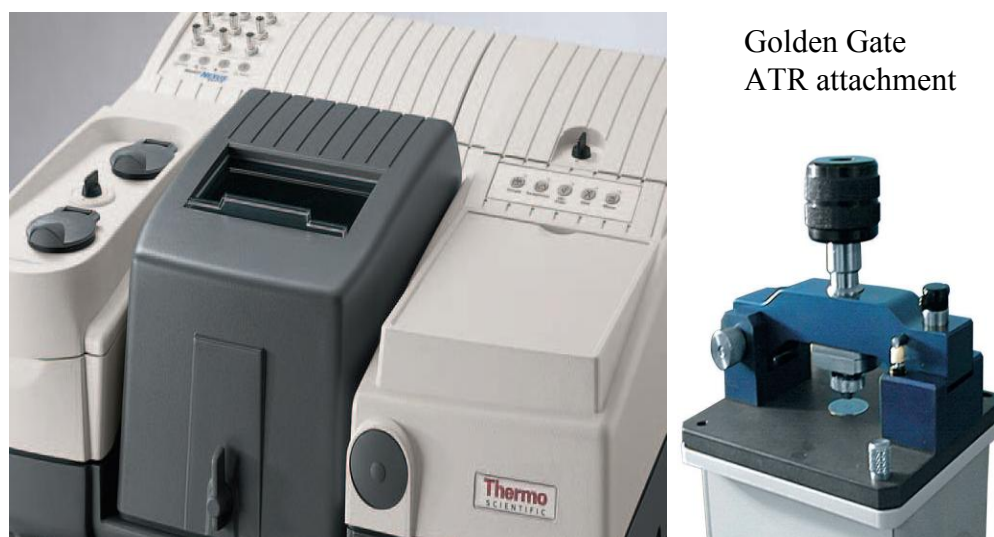
Figure 4.6 Nicolet 8700 FTIR spectrometer (left) with Golden Gate ATR attachment (right)
