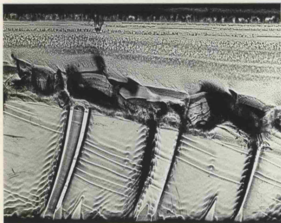
Figure 9.4 Rib marks with crazed zone on immersed (stick-slip) sample. X13.
