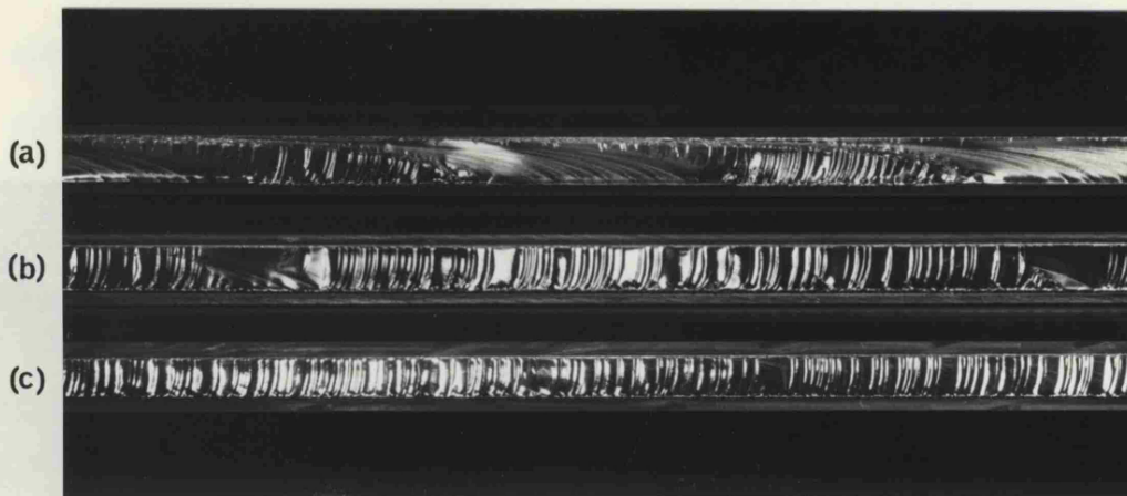
Figure 11.8 Fracture surfaces : grease coated PMMA samples with a blunt starter crack, immersed in distilled water. Cross-head speeds (a) 0.2 (b) 0.5 (c) 1.0 mm/min.
