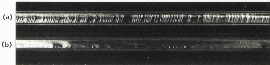
Figure 9.15 Fracture surfaces of immersed samples, cross-head speed 50 mm/min.
