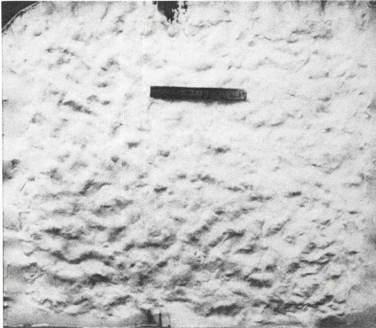
Fig 2 Model Rough Surface With Six Inch Ruler Showing Scale
