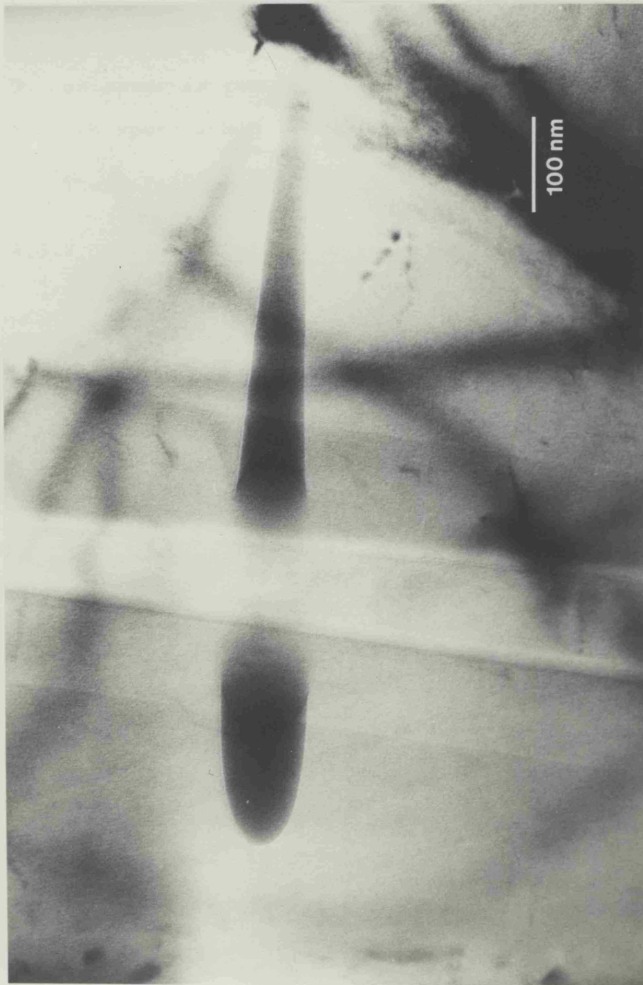
Fig. 40 Projected width of a slip trace and corresponding contamination spot displacement (stainless steel foil).
