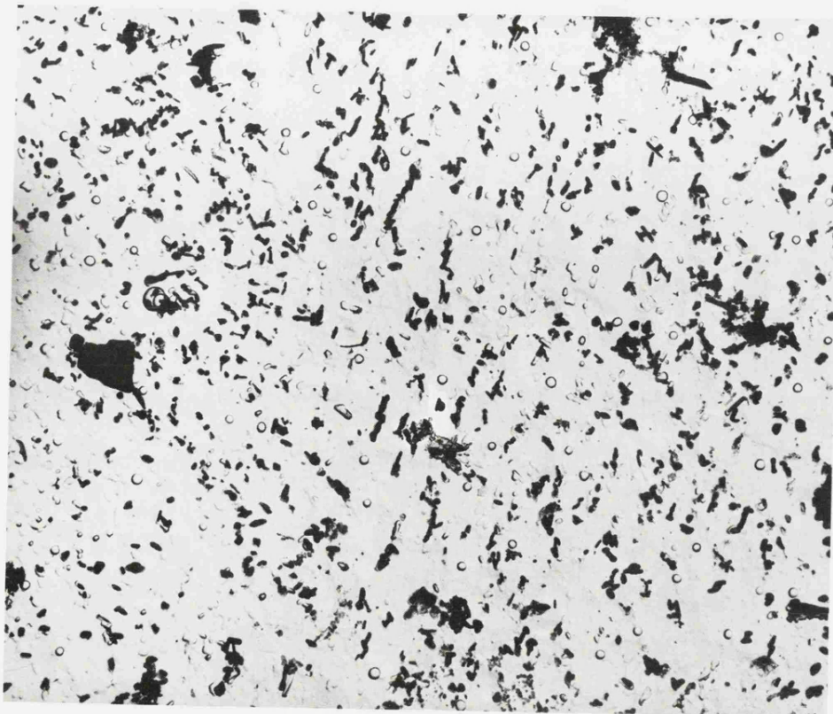
FIGURE 31 EXTRACTION REPLICAS OF THE STRUCTURE PRIOR TO TEST. X 5,600 TOP BATCH 1, BOTTOM BATCH 2.
