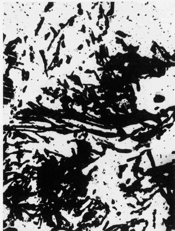
FIGURE 30 FORMS OF CARBIDES IN PEARLITE. EXTRACTION REPLICAS. X 5,600
