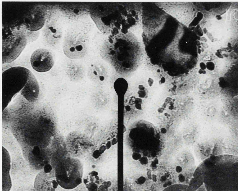
FIGURE 28 SELECTED AREA DIFFRACTION FROM THE SMALL AREA SHOWN. X 30,000 THE LOWER PHOTOMICROGRAPH SHOWS THIS AREA IN DETAIL. X 100,000 SHADOWED REPLICAS.
