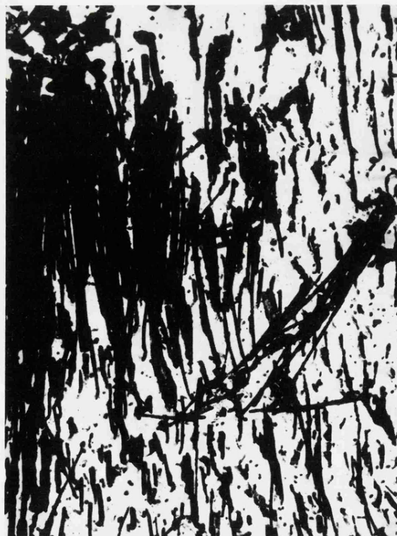
FIGURE 30 FORMS OF CARBIDES IN PEARLITE. EXTRACTION REPLICAS. X 5,600
