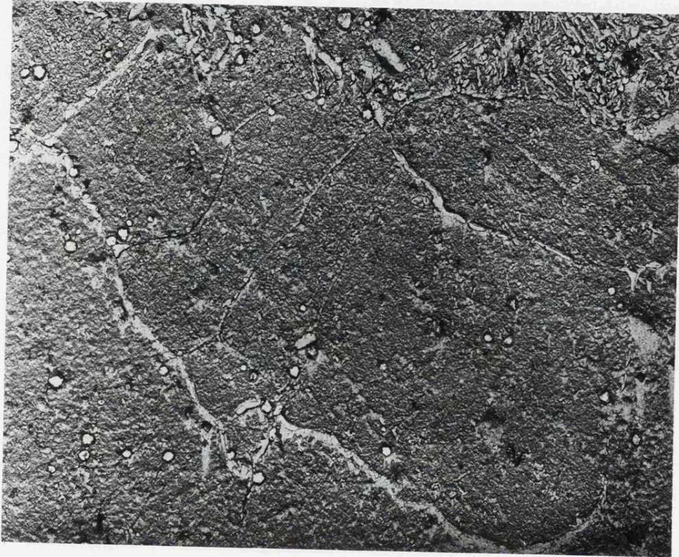
FIGURE 27 SHADOWED REPLICA SHOWING GRAINBOUNDARY MIGRATION. X 1,600
