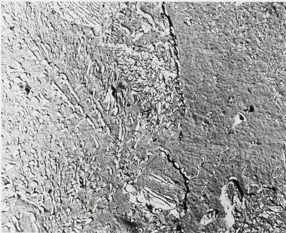
FIGURE 26 SHADOWED REPLICAS OF THE MICROSTRUCTURE PRIOR TO TEST. X 1,600 TOP BATCH 1, BOTTOM BATCH 2
