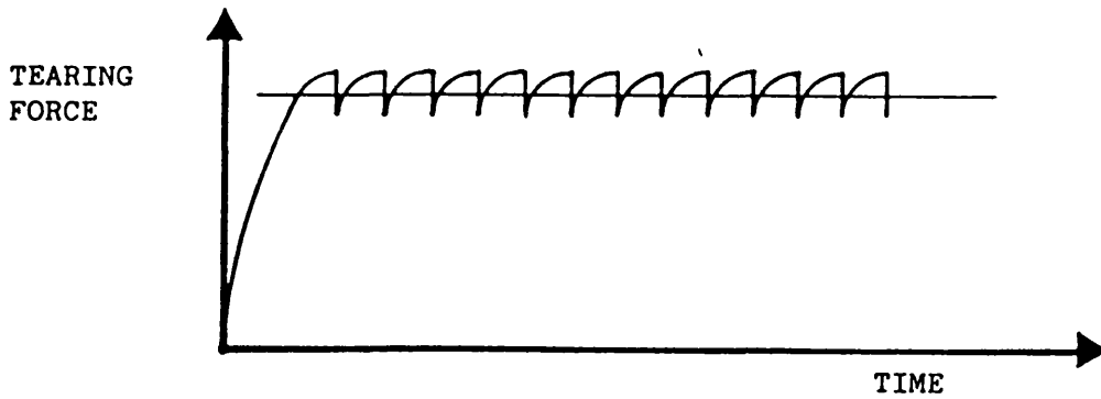
FIGURE 5-7 : Copy of a tearing force - time trace for E.V.A. copolymers.
