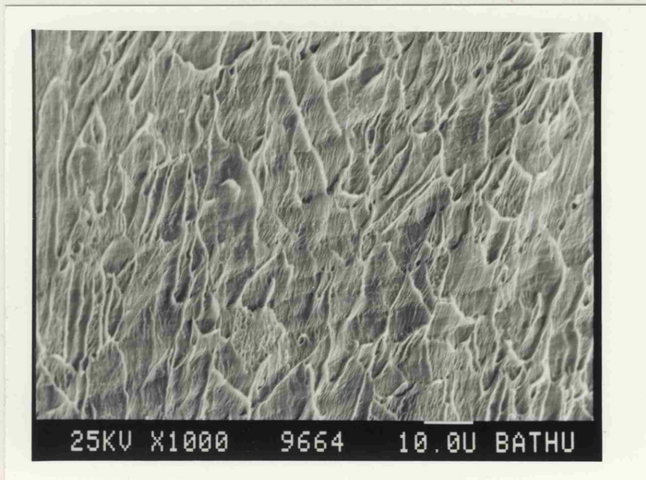
PICTURE 2: Backed polymer B peeled from chemically polished copper (polymer side). Peel load 2.09 \text{ N.mm}^{-1}
