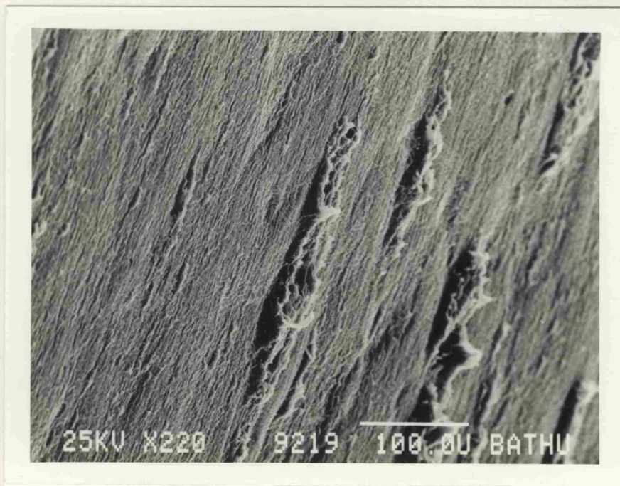
PICTURE 10: Unbacked polymer A peeled from etched steel (polymer side). Peel load 3.03 \text{ N.mm}^{-1}
