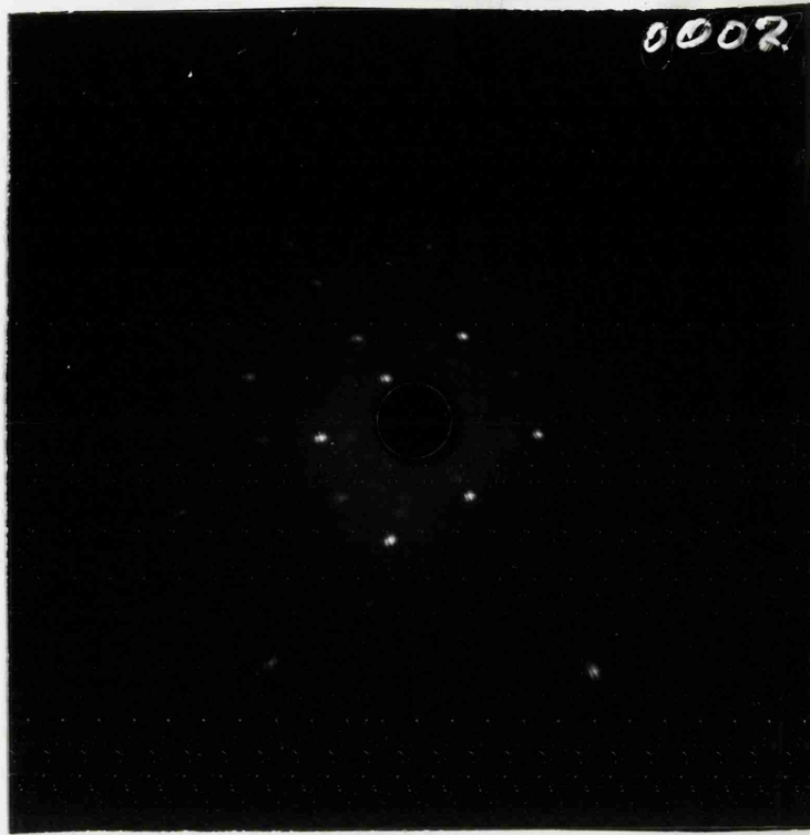
Figure (4.6) Laue-reflection X-ray photograph of antimony along the binary ( x ) axis.
