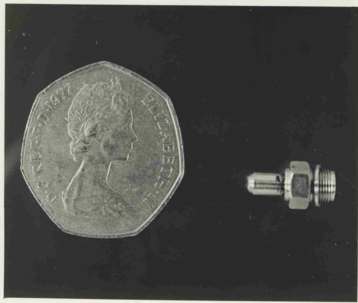
Fig. 3.1 Piezoelectric pressure transducer used for fluid borne noise tests
