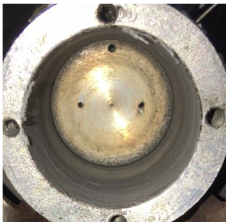
Figure 5a. Test 1 post firing aluminium combustion chamber (no damage)
