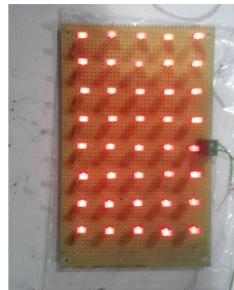
Figure 3b. LED distribution behind the panel
