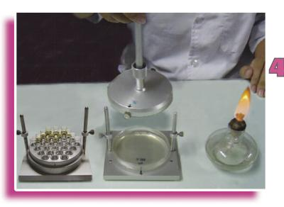
the apparatus Set ensure that the surface of each multiple inoculator stick will properly touch the surface of the medium in agar plate.
