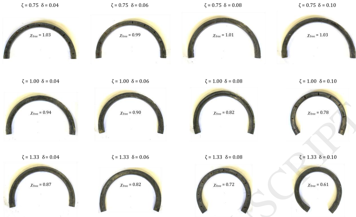
Fig 16 Experimental results for free curvature change in ring rolling of half rings for various tool size ratios ( \zeta ) and reductions in thickness ( \delta )
