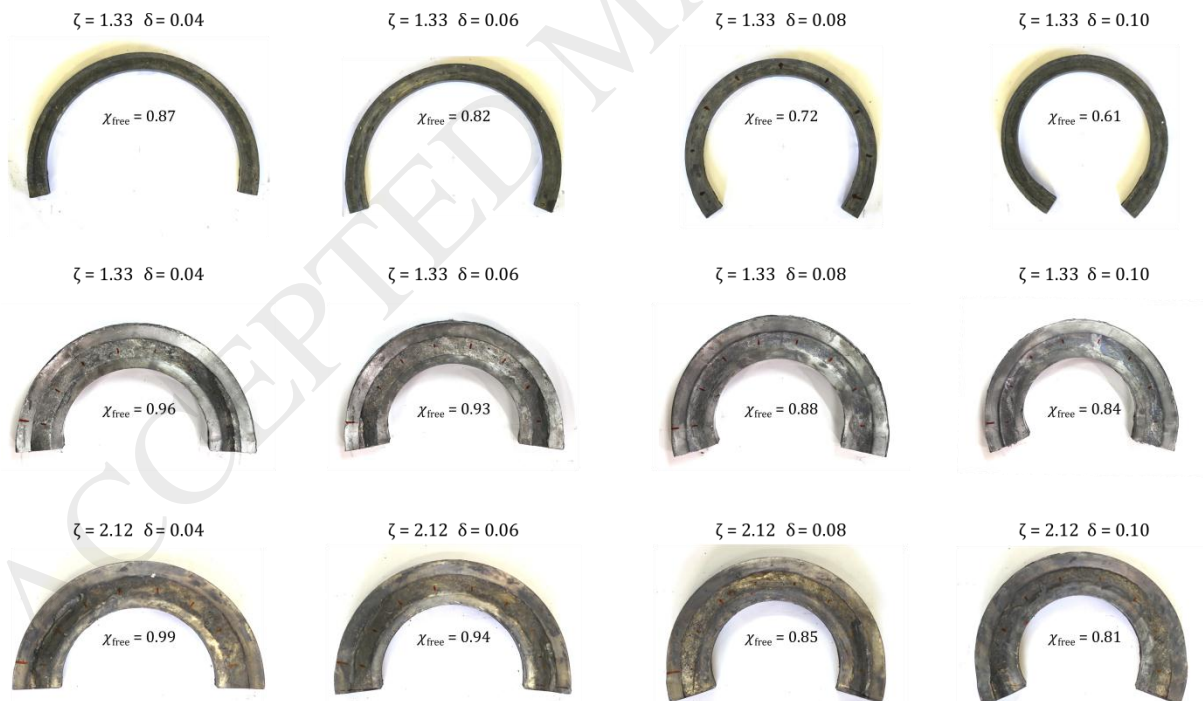
Fig 17 Comparison of free curvature change for medium-walled and thick-walled half rings, with tool size ratio \zeta = 1.33 and 2.12 , varying the reduction in thickness ( \delta )
