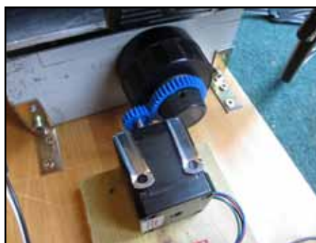
Fig. 4. Plastic gears driving the fine focus knob.
