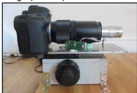
Fig. 1. The rail based on an old microscope.
