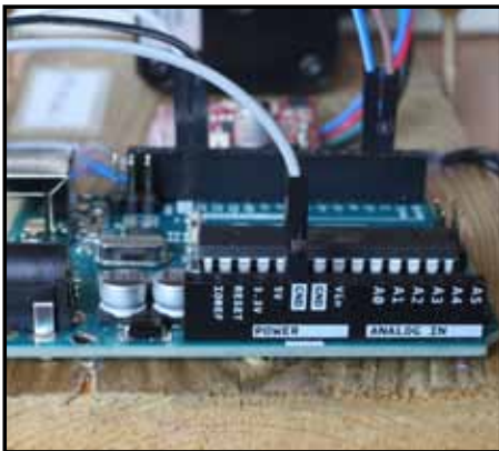
Fig. 8. The wiring for the Arduino showing the driver wires right and centre.
