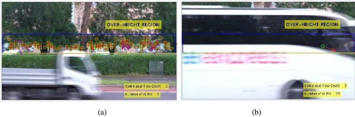
Fig. 5 Two instances in which the algorithm did not pick up sufficient features to track adequately for five frames or more. (a) and (b) The vehicle did not pass trigger#2 (average displacement of pixels over threshold limit) and therefore is missed as an OHV
