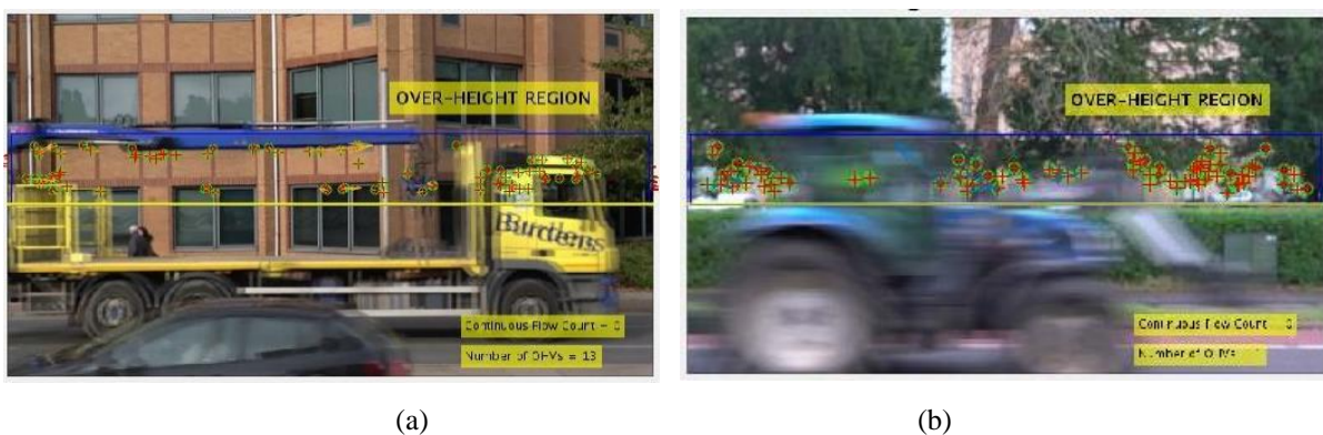
Fig. 4 (a) shows an instance when insufficient features are tracked on the vehicle to pass triggers #2 and #3; (b) shows a tracker vehicle in the scene. Out of the 5 feature detectors, only SURF could reliable track the vehicle over 5 frames consecutively. The other feature detectors failed in this instance
