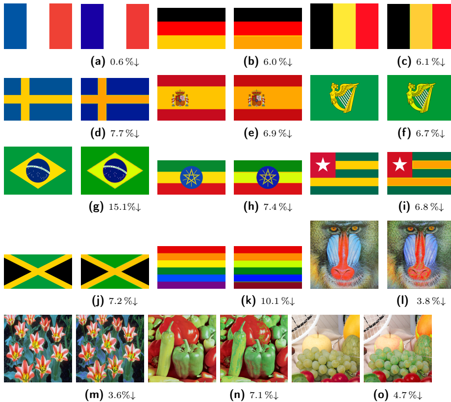
Figure 5. Outputs of Ishihara programs before transforms (left image in pair) and after perceived-color program transforms with p_{\pi} = 0.01 (right image in pair). The captions within the figure show the difference in OLED display power dissipation between the two images in each pair. The pairs look similar to many observers when viewed on a standard LCD or OLED display.
