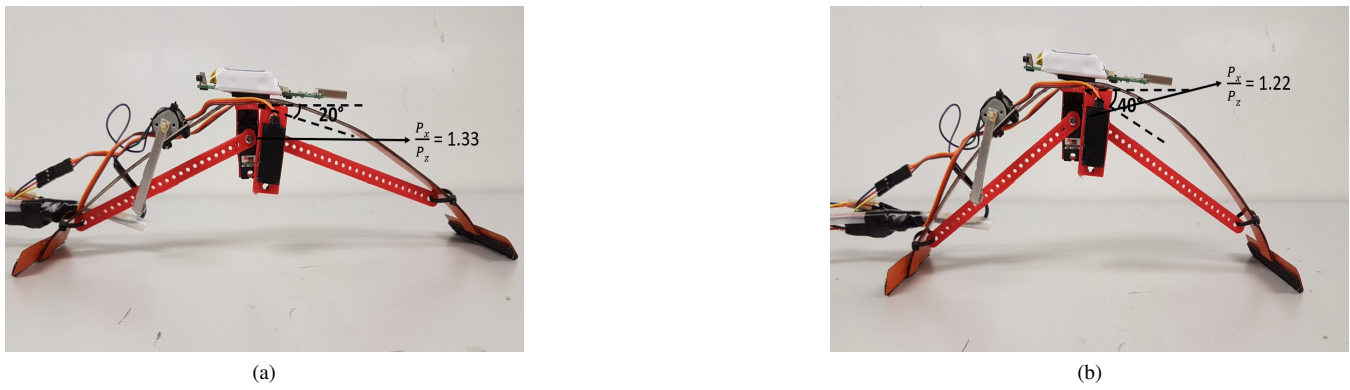
Fig. 7: Inverted U-shape curved beam robot in two different configuration indicating acting dominant forces that drive the locomotion through the ratio of the power coefficients. (a) When the robot is in the horizontal position, its tendency is to slide forward with power in x axis dominating the power in the z axis. (b) And, when the robot is in upright position it has more tendency to diagonally hop forward as the power in x axis and z axis are more balanced. The ratio P_x/P_z shown here is taken from the results shown in Figure 6.
