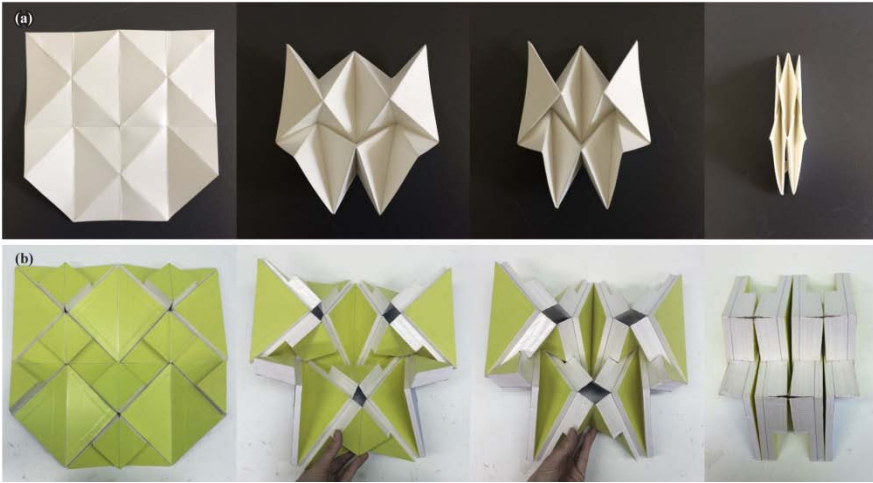
Figure 4: Waterbomb pattern.(a) Paper model. (b) Origami of thick panels.
