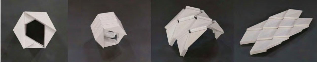
Figure 1: Origami of thick panels by Chen, Peng and You (diamond origami pattern). Hexagonal elevation and deployment sequence.
