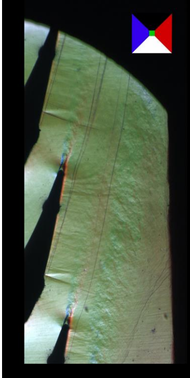
Fig. 24 – Schlieren image of the 16.2% of throat Elliptical trailing edge blades in the Cascade Rig, at M_{2,mix} = 0.90 , Re_2 = 2.6 \times 10^6 .
