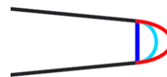
Fig. 6 – Comparison of Square, Round and Elliptical trailing edge geometries tested in the Isolated Trailing Edge Rig.
