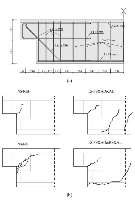
Figure 8: Experimental program: (a) Specimen geometry and reinforcement lay-out, (b) developed crack pattern at 175 kN load mapped to the proposed defect zones
