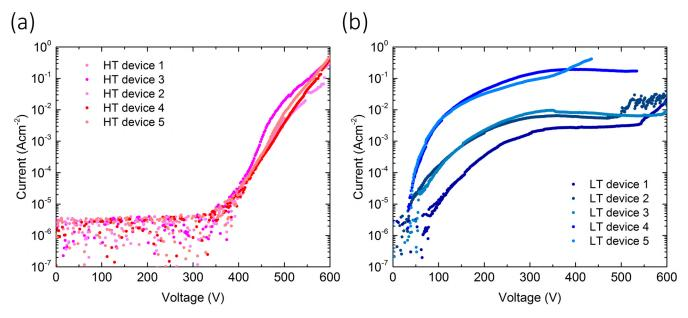
FIG. 2. Vertical leakage current of the (a) HT sample and (b) LT sample with bias ramping from 0 V to 600 V. It can be seen that the vertical leakage currents in the LT sample are significantly higher and more variable than the HT sample.
