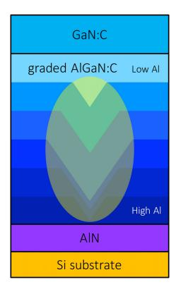
FIG. 9. Schematic diagram showing the evolution of the growth front of a V-pit opening up at the beginning of the AlGaN SRL growth, then closing up as the growth temperature is increased and the Al composition is decreased. Eventually, a planar surface is recovered at the end of AlGaN SRL growth. Preferential incorporation of oxygen on the semi-polar sidewalls of the V-pit gives rise to the formation of a conductive pathway in the AlGaN SRL as indicated by the light green shaded area.
