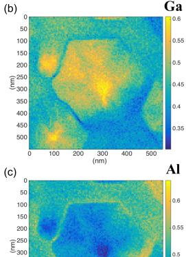
FIG. 8. A hexagonal defect in the middle of AlGaN SRL of the LT sample with (a) annular dark field STEM image (b) Ga and (c) Al composition images from EDX analysis. The composition images show that the defect is Ga-rich and Al-deficient at its centre.
