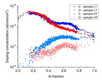
FIG. 6. Carbon and oxygen concentrations vs Al fraction in the AlGaN SRL of the LT and HT samples from SIMS measurement. The LT sample (blue) shows a higher carbon level in the bottom half of SRL than the HT sample (red). The oxygen level in the LT sample is always higher than that in the HT sample.
