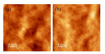
FIG. 4. AFM image of surfaces for (a) LT and (b) HT samples. The image size is  $20 \times 20 \,\mu\text{m}$ . The colour scale is  $10 \,\text{nm}$ . The root mean square of surface roughness  $R_q$  is (a)  $1.08 \,\text{nm}$  and (b)  $1.05 \,\text{nm}$ .
