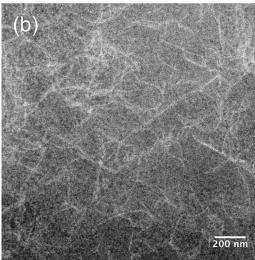
FIG. 7. Annular dark field STEM images of the (a) LT sample and (b) HT sample. Hexagonal defects were only found in the LT sample but not the HT sample. A defect labeled with yellow arrows has misfit dislocations clustering at the centre.
