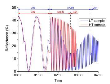
FIG. 3. 635 nm reflectance signal during growth for the LT and HT samples. The LT sample shows a significant decrease in the reflectance signal in the middle of the AlGaN SRL in contrast to the HT sample.
