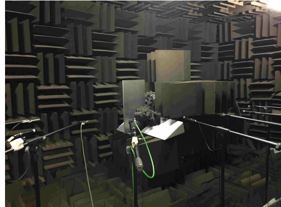
(b) The installed jet noise experiment setup: microphones are located at 50D to the jet nozzle centre on the shielded side, with observer angle ranging from 30^\circ to 120^\circ to the jet centreline.
