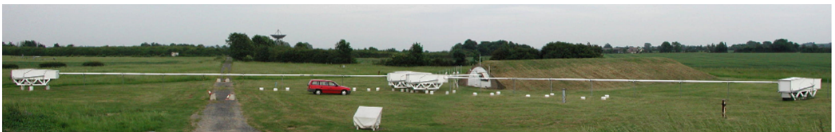
Figure 1.5.: COAST in profile; visible in this photograph are the 5 array telescopes (3 are located together at the centre of the picture), the laboratory bunker, and the light propagation pipes.
