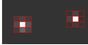
Figure 5.16.: One frame from the shuffled charge imaging mode. The grids represent the 3 \times 3 grid used for calculating difference signals.
