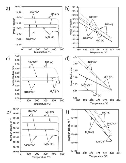
**Figure 12.** Precipitation kinetic in martensite during cooling from austenitisation; (a)–(b) phase fraction; (c)–(d) mean radius; (e)–(f) number density versus time.
