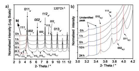
Figure 3. (a) X-ray diffractogram of HT10, austenitised and cooled at 120° Ch<sup>-1</sup>; (b) magnified section of (a).
