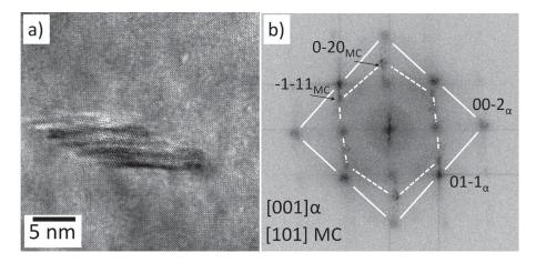
**Figure 7.** Small MC precipitate observed after slow-cooling from 1050°C and tempering at 600°C for 24 h; (a) HRTEM image (b) FFT diffractogram of (a) showing that the alloy carbide possesses Baker and Nutting orientation relationships with martensite lath.
