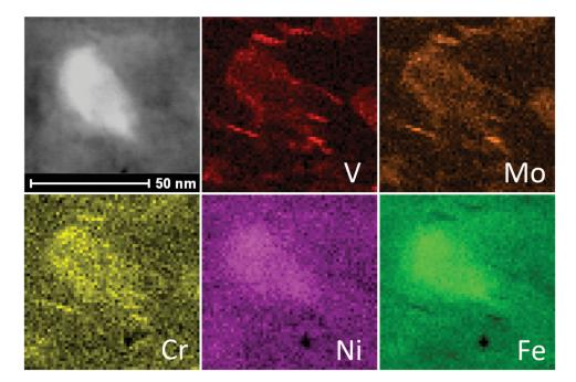
**Figure 9.** Fast-cooled sample, tempered at 600°C for 10 h. Cr, Ni, Fe-rich precipitates with some V, Mo, Cr carbide. The Cr, Ni, Fe-rich precipitation is austenite ( $\gamma'$ ), while V, Mo, Cr-rich precipitate is carbide.
