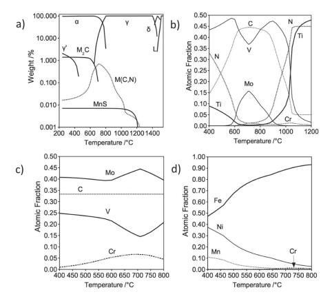
**Figure 15.** (a) Equilibrium phase weight per cent of HT10 as a function of temperature. (b)–(d) The atomic fraction of (b) M(C,N), (c)  $M_2C$ , (d) austenite ( $\gamma'$ ) as a function of temperature.
