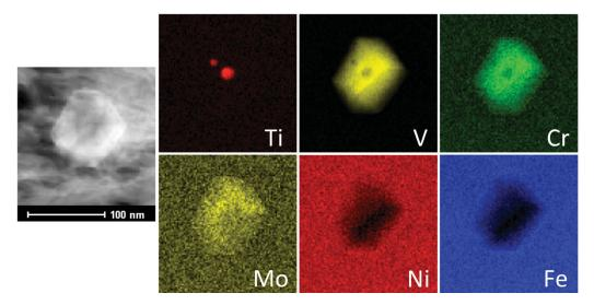
Figure 10. Ti-rich particle encapsulated by V, Mo and Cr following slow-cooling (120°C h<sup>-1</sup>).
