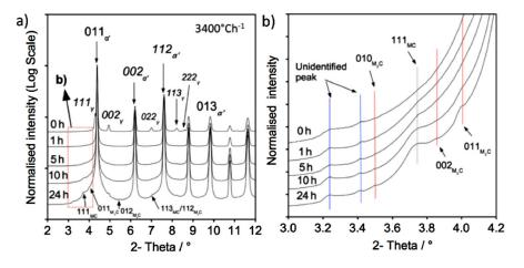
**Figure 2.** (a) X-ray diffractogram of HT10, austenitised and cooled at  $3400^{\circ}$  Ch<sup>-1</sup>; (b) magnified section of (a).
