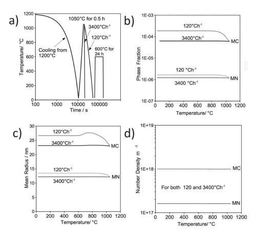
**Figure 11.** (a) Heat treatment cycle used for the simulation. (b–d) Precipitation kinetic in austenite during cooling from austenitisation; (b) phase fraction, (c) mean radius and (d) number density.
