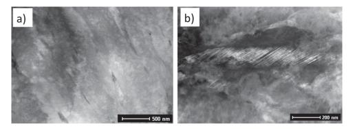
Figure 6. Microstructures following slow-cooling (120° Ch<sup>-1</sup>); (a) lath martensite matrix, (b) twin martensite.
