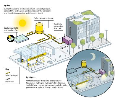
works toward a carbon-free hydrogen fuel that can be used in a fuel cell, an electrochemical engine that is inherently more efficient than the internal combustion engines we use with fossil fuels [10].
