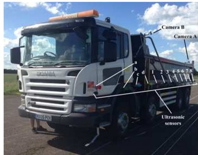
Figure 2. Camera and ultrasonic setup
