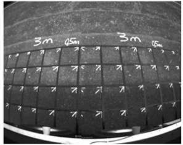
Figure 9. Calibration grid processed to cover the entire image
