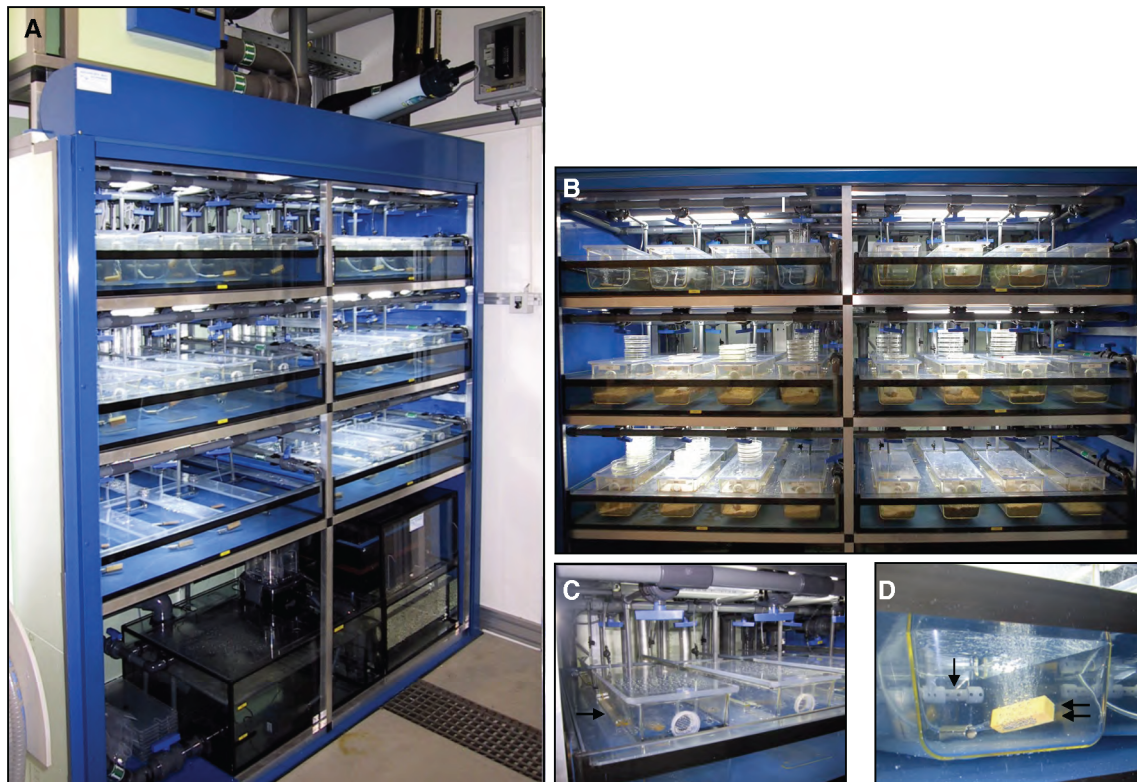
Figure 1. The amphioxus facility. (A) Lightproof cabinet of the facility, with open shutters, showing three shelves with two main tanks each. The upper distribution tank and UV sterilisation device are visible at the top outside the cabinet. The two-compartment lower reservoir tank and neighbouring filter unit are at the base of the facility inside the cabinet. (B) View of the six main tanks encapsulating eight amphioxus boxes each, distributed in two rows of four. All tanks in use are sand-bedded. (C) Encapsulated tank system: the amphioxus boxes are encapsulated into the main tank through a fitted PVC grid (arrow), leaving two thirds of their height immersed in the main tank. The unique unsealed part is the netted outlet (double arrow) of the amphioxus boxes, used for the flow-through circulation of the seawater. (D) All amphioxus boxes are equipped with inverted T-shape water jets, multi-perforated at the base (arrow). This was conceived to generate a unidirectional seawater wave washing out the entire width of the boxes. In addition, all amphioxus boxes are equipped with 5 cm air stones (double arrow) to constantly oxygenate the water by dispersion. doi:10.1371/journal.pone.0071599.g001
