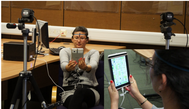
Figure 3. Participant shown with OptiTrack marker setup and engaging with the map application used in Experiment 1 and 2 (inset).
