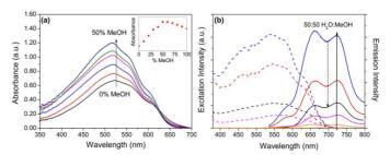
**Figure 5.** (a) UV/Vis absorption spectra of **P3HT-***b***-P3HTPy** in H<sub>2</sub>O/MeOH solvent mixtures. Inset: Absorbance at 522 nm ( $\lambda_{max}$ ) as a function of Vol% MeOH in H<sub>2</sub>O/MeOH mixtures. (b) Selected excitation ( $\lambda_{em}$  = 730 nm) and PL ( $\lambda_{ex}$  = 515 nm) spectra of **P3HT-***b***-P3HTPy** in 100% MeOH (orange line), 70% MeOH (violet line), 50% MeOH (blue line), 30% MeOH (red line) and 0% MeOH (black line).
