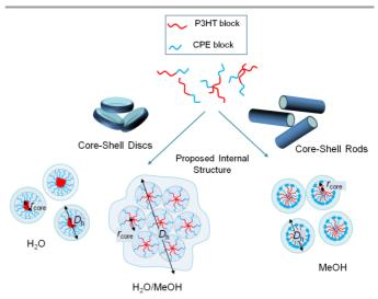
**Figure 9.** Schematic representation of the proposed internal aggregate structures for **P3HT-b-CPE** in  $H_2O$ , MeOH and  $H_2O$ /MeOH mixtures.  $L_{core}$ ,  $r_{core}$  and  $T_{shell}$  are the core length, core radius and shell thickness obtained from SANS data fitting, respectively.  $D_h$  is the hydrodynamic diameter measured by DLS. We note that the precise arrangement of the P3HT and CPE block domains in the aggregates formed in MeOH is still undetermined.
