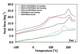
Figure 2. RHC thermogram of P3HT-b-P3HTPMe<sub>3</sub>, showing the first heating (red) and the second heating (black). After storage at ambient conditions a curve similar to that of the first heating is found (blue). Thermograms of the second heating and after storage at ambient conditions are also included for pure P3HTPMe<sub>3</sub> for comparison (dashed and solid green). The curves were shifted vertically for clarity.
