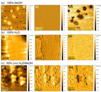
**Figure 8** AFM tapping mode images of **P3HT-b-P3HTIm** films drop-cast from (a) 100% MeOH (7  $\mu$ g mL<sup>-1</sup>), (b) 100% H<sub>2</sub>O (3.5  $\mu$ g mL<sup>-1</sup>) and (c) 50% (v/v) H<sub>2</sub>O/MeOH
