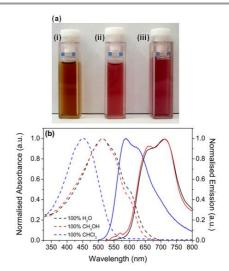
**Figure 4.** (a) **P3HT-b-P3HTPMe**<sub>3</sub> in (i) CHCl<sub>3</sub>, (ii) MeOH and (iii) H<sub>2</sub>O. (b) Corresponding normalised UV/Vis absorption and emission spectra for **P3HT-b-P3HTPMe**<sub>3</sub> in 100% CHCl<sub>3</sub> (blue), 100% H<sub>2</sub>O (black) and 100% MeOH (red).
