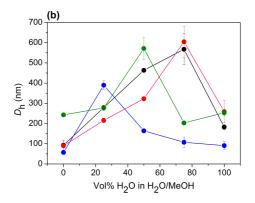
**Figure 6.** (a) Fluorescence quantum yields ( $\Phi_F$ ) and (b) hydrodynamic diameter ( $D_h$ , Z-average) of **P3HT-b-CPEs** in H<sub>2</sub>O/MeOH solvent mixtures (0.35  $\mu$ g mL<sup>-1</sup>). Legend: **P3HT-b-P3HTPy** (blue circles), **P3HT-b-P3HTIm** (black circles), **P3HT-b-P3HTNMe**<sub>3</sub> (red circles) and **P3HT-b-P3HTPMe**<sub>3</sub> (green circles).
