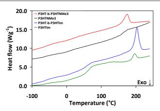
Figure 3. RHC thermogram of P3HT-b-P3HTNMe<sub>3</sub> (red) and P3HT-b-P3HTIm (blue), showing the second heating. For comparison the second heating of the P3HTNMe<sub>3</sub> (black) and P3HTIm (green) pure polymers is shown. The curves were shifted vertically for clarity.
