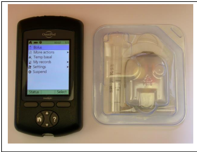
Fig. 1. Insulet OmniPod system: PDM and Pod.
