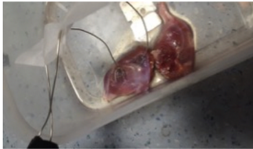
1) Photograph of the experimental set up. Rat lower limb muscle with field stimulation electrodes (left), control muscle without stimulation electrodes (right).
