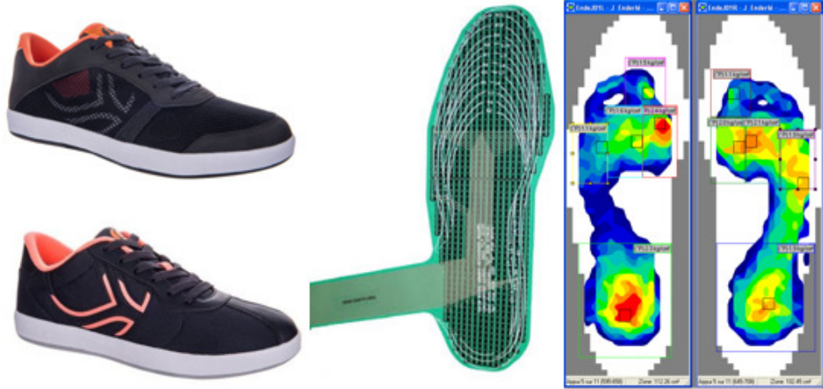
Figure 1. Footwear used and F-Scan® in-shoe pressure measurement insoles along with manual mapping of foot regions. Left image top – male model and bottom – female model.
