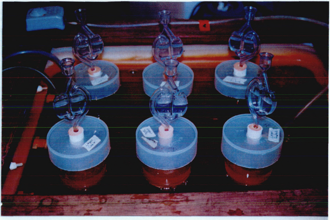
Fig 2.1 Static wort fermentations in 1L Imhoff cones (Nalgene) at 18°C in a circulating water bath.
