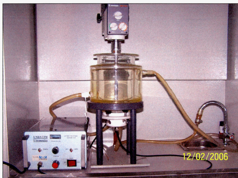
Figure 2.5: High frequency (520 kHz) US reactor with an overhead stirrer (200 rpm) (Bogazici University, Turkey).
