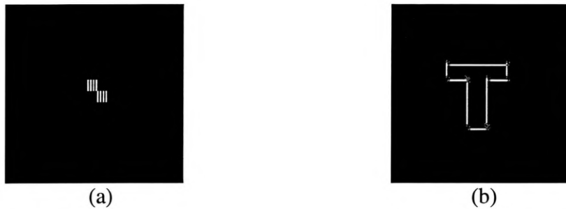
Fig. 7.9 Computer simulation result with Roberts gradient: (a) the encoded Roberts gradient, and (b) the correlation result of the letter 'T' with Roberts gradient.
