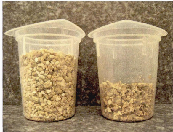
Figure 2-1: Vermiculite untreated (left) and washed in \text{CaCl}_2 -solution (right), weight 10 g of air dried vermiculite.
