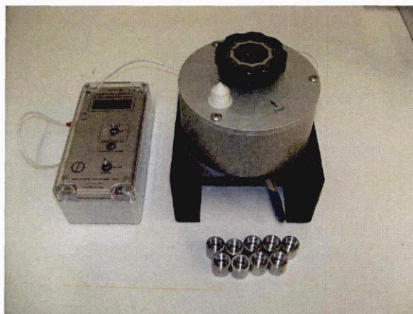
Figure 2-4: Tru Psi thermocouple psychrometer (Decagon Devices) with 9 sample holders (metal cups).
