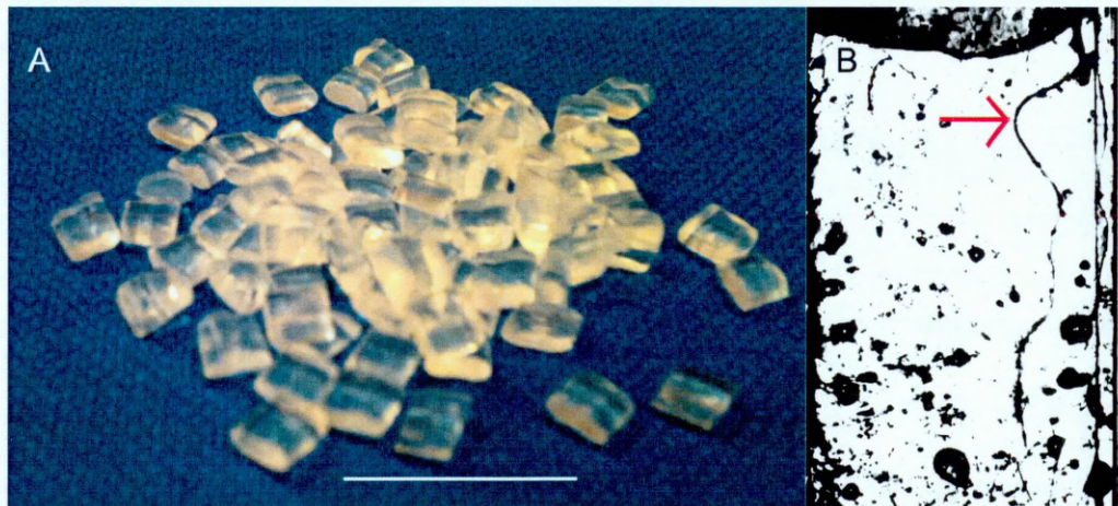
Figure 2.3. FEP - a candidate material for constructing a transparent substrate. A) Granulates of FEP in its unprocessed form. Scale bar = 1 cm. B) Root imaging was achieved in an FEP-based, saturated, RI matched substrate. Red arrow indicates the root.
