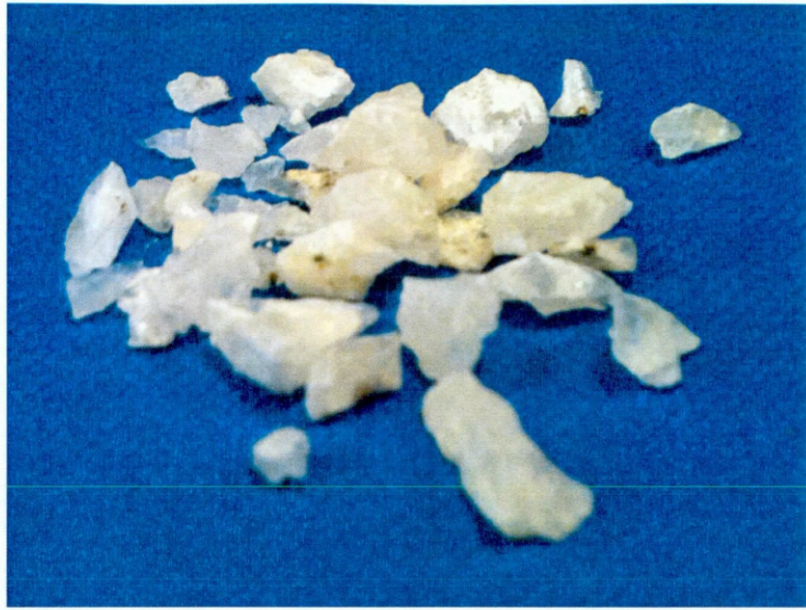
Figure 2.2. Particles of the mineral cryolite – a candidate material for constructing a transparent, granular, RI matched substrate. Scale bar = 1 cm.
