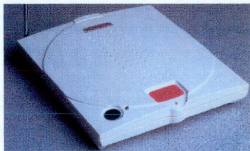
Figure 3.7: The replacement community alarm
