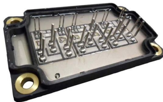
Fig. 1. Multi-chip layout of SiC MOSFET power module [3]
